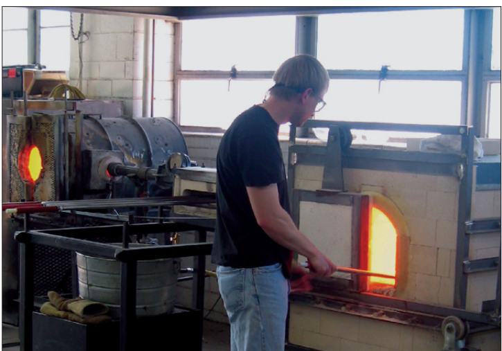
Photo by Ann Bierbower Paul Engler, senior, who has blown glass for five years, rotates a steel rod inside the 2,000° "glory hole" as glass melts on the other end. This is the beginning of what will become a 12 inch vase.
