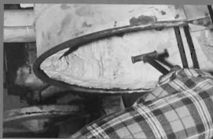
Halva taps a work of glass directly into the lehr.
